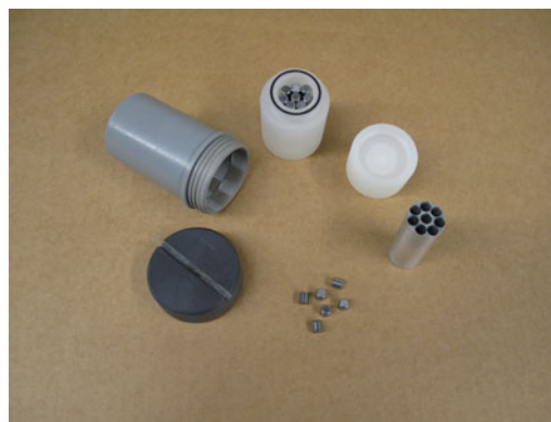
Figure 4. Miniaturized-grinding vessel for a McCrone Micronizing Mill. Clockwise from top center: white polypropylene vessel base loaded with tungsten carbide rods and O-ring, vessel lid, aluminum loading device, loose tungsten carbide rods, hardened polyvinyl chloride lid, and gray polypropylene jar.
