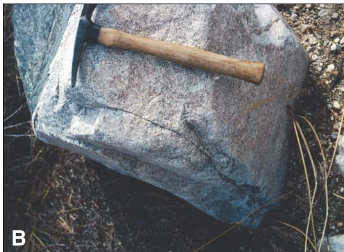
Figure 4. Photographs of the 4 primary crack types observed in this study (see text for further explanation). (A) Fabric-related cracks, including cracking ranging from thin to separated. (B) Surface-parallel crack that is not a spall. (C) Longitudinal crack. (D) Meridional crack.
